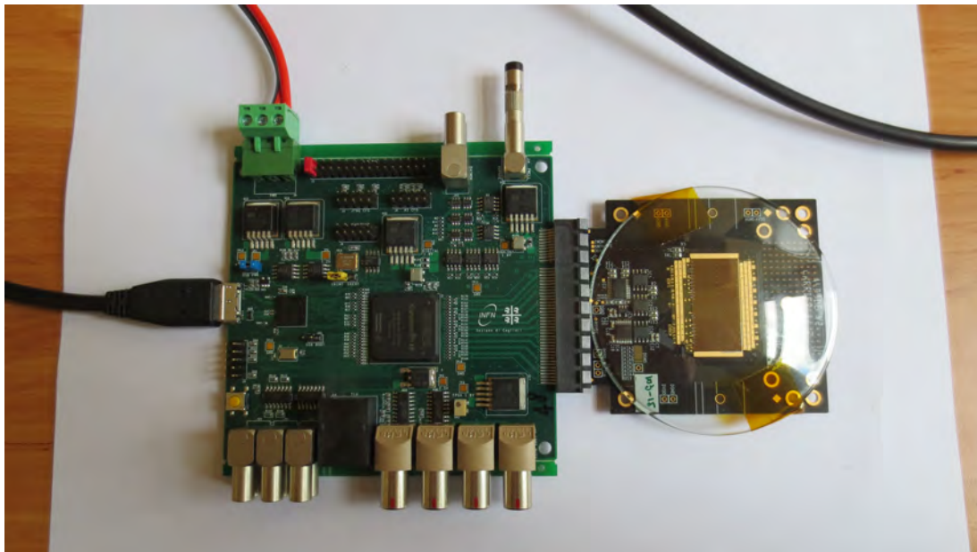
Figure 3.2: Setup for performing tests of the pALPIDEfs chips. The chip carrier on the right with the chip in the middle of it and covered by glass is connected to the operating electronics on the left. A USB port providing connectivity with a notebook is connected to the left side of the operating board. The power supply cable can be seen connected at the top.
