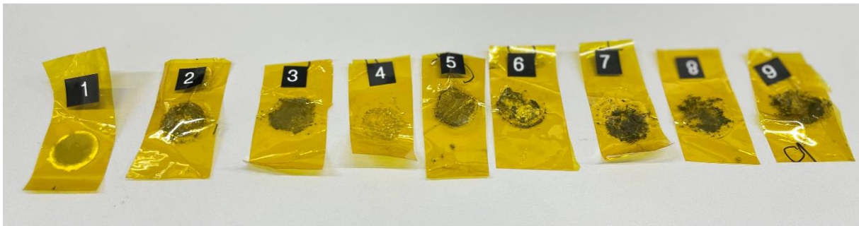
Figure 1: Photo of the prepared Sn-coated aluminium electrodes. The pulverization is clearly visible in all the samples (number 2-9). The uncoated pristine aluminium electrode (number 1) is the only sample in a solid state.
