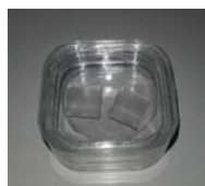
Figure 1: The polycarbonate blocks of 10 x 10 mm and a thickness of 3 mm cut with a diamond disc and subsequently cleaned with an ultrasonic cleaner
