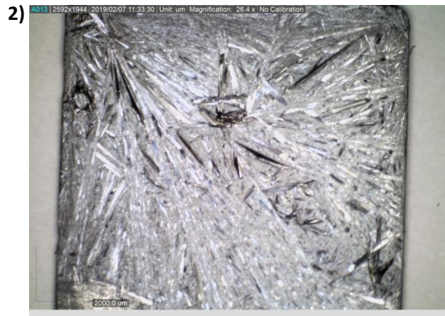
Figures The evolution of V-SANS curves (high-resolution mode) in 0.15 wt.% Ti sample (1) and the surface of sample after sintering experiments (2 and 3).
