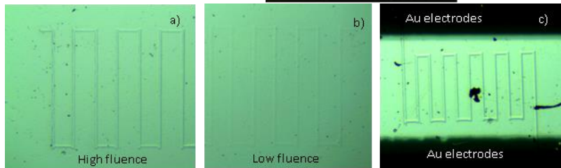
Fig. 2. Optical images resistors written at 3.8 \cdot 10^{13} ions/cm 2 a) at 3.7 \cdot 10^{14} ions/cm 2 b) a resistor written between two electrodes at 3.7 \cdot 10^{14} ions/cm 2 c) all written in PMMA.
