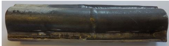
Fig. 1: Circumferential test weld of 7 CrMoVTi10-10 creep resistant steel
