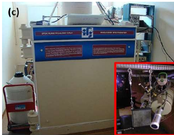
(a) NCSR D 85% relative efficiency HPGe coaxial detector and (inset) detector shown inside low background configuration; (b) CCFE BEGe detector and cryogenic recycler with (inset) Nal Compton suppression ring inside a Pb/Sn/Cu low background shield; (c) Whole-body spectrometer at IFJ PAN view from outside low background shielding, and (inset) a pair of 30% relative efficiency HPGe detectors inside the shielding separated by a suspended lead shield; (d) ENEA HPGe detector inside low background shield.
