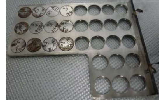
LTIS assembly tray post-irradiation, with some dosimetry foils removed
