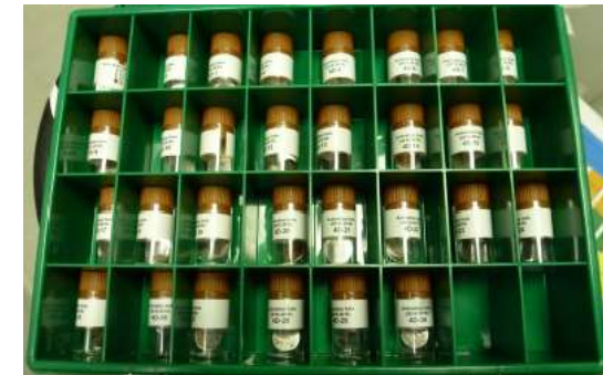
Collected activated dosimetry foil samples from 4D, prior to distribution and measurement analyses.
