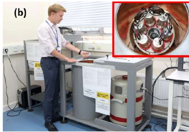
LTIS assembly tray post-irradiation, with some dosimetry foils removed
