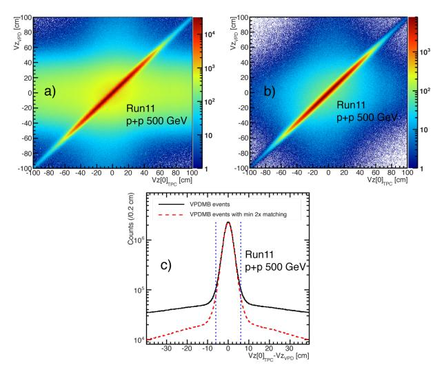
Figure 3.2: Correlation between z-position of the first TPC vertex and z-position of the VPD vertex from VPDMB trigger before (Panel a) and after (Panel b) 2x matching in Fast cut is applied. Panel c): Vertex z-position difference between the TPC vertex and the VPD vertex. The blue vertical lines indicate the cut window used to select the triggered events.
