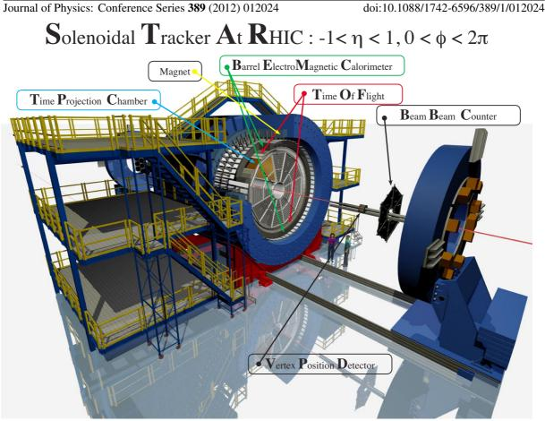
**Figure 1.** The STAR detector. TPC (Time Projection Chamber) is main detector for tracking and PID (provides  $dE/dx, \vec{p}$ ), TOF (Time Of Flight) is used for PID improvement and pileup tracks removal, BEMC (Barrel Electromagnetic Calorimeter) used for electron identification improvement and pile-up tracks removal.
