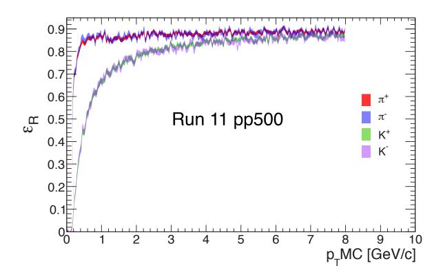
Figure 4.1:  $\pi^+, \pi^-, K^+, K^-$  track reconstruction efficiency. Errors are depicted by contours.
