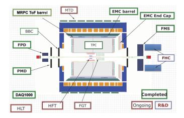
Figure 1: The STAR detector. TPC (Time Projection Chamber) is main detector for tracking and PID (providing dE/dx,  $\vec{p}$ ), TOF (Time Of Flight) for PID improvement, and pile-up tracks removal and BEMC (Barrel Electromagnetic Calorimeter) in this analysis for pile-up tracks removal if TOF is not available.
