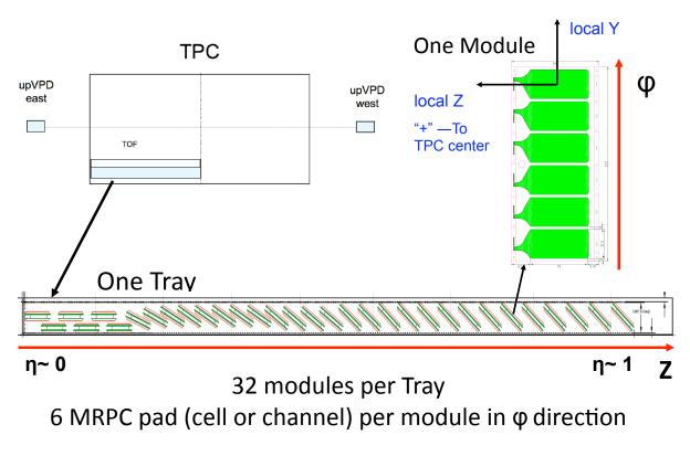
Figure 2.8: Barrel Time Of Flight geometry.
