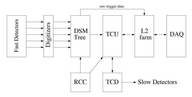
Figure 2.3: The STAR Trigger.
