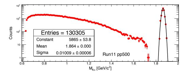
Figure 3.12: Invariant mass spectrum of oppositely charged kaon-pion pairs. Kaons pions came from  $D^0$  hadronic decay generated by PYTHIA and their momenta were randomly smeared by gaussian functions with widths equal to known  $p_T$  resolution values.
