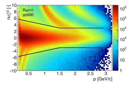
Figure 3.8:  $n\sigma_{\pi}^{1/\beta}$  as a function of the track momentum. The black lines depict the TOF PID cut for pions.  $1/\beta$  of pions is affected by Coulomb re-scatterings at lower momenta so I used a wider range according to (3.6).
