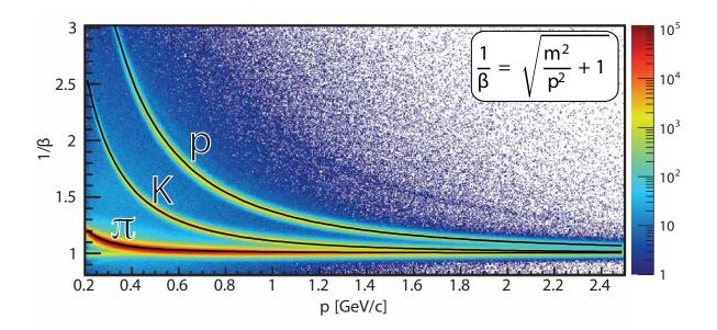
Figure 2.10: Particle Identification by STAR TOF.
