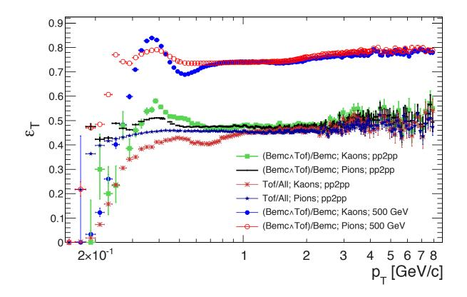
Figure 4.2: TOF Matching efficiency as a function of the track  $p_T$ . Open red (closed blue) circles depict the efficiency calculated according to (4.3) from the production P11id for pions (kaons). The pp2pp data were analyzed 1) by the same way with results depicted as green closed squares (kaons) and black thick dots (pions) 2) according to (4.4) with results depicted as dark red crosses (kaons) and dark blue (pions) asterisks.
