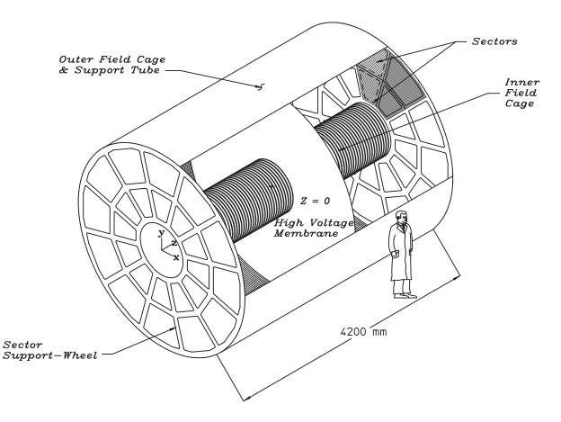
Figure 2.4: The STAR Time Projection Chamber.
