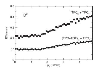
FIG. 9. Total  $D^0$  reconstruction efficiency versus  $D^0 p_T$ .
