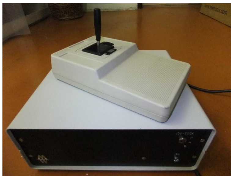
Figure A.3.1 – The MCL-2 control module with manual control joystick
