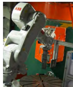
robotic arm for sample positioning
