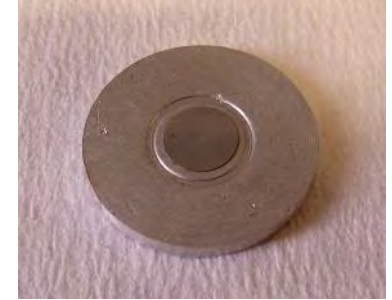
Cold pressing for powders, e.g. ^{100}\text{Mo}
