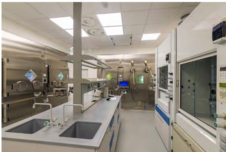
Fig. 8 Radiochemical laboratory over the cyclotron TR-24 – a view on the four hot cells and two radiochemical fume hoods intended for target processing, separations and labellings.
