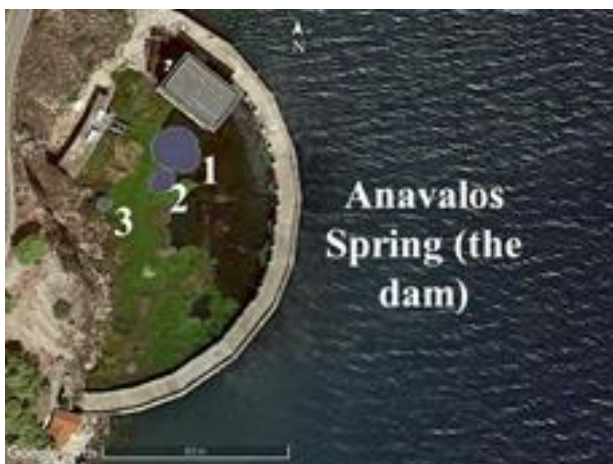
Figure 1. The dam surrounding the SGD spring of Anavalos. The main three “eyes” of the freshwater discharges are mentioned with blue. The aquatic plants grown in the dam are shown with green.
