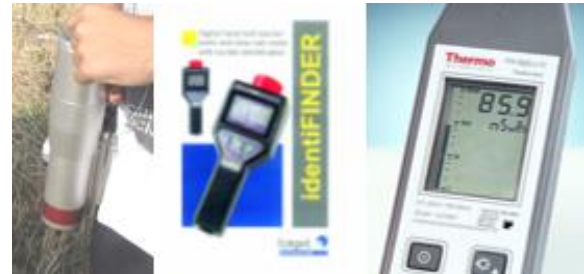
Figure 1. Portable detectors used for the in-situ survey.
