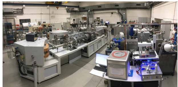
Figure 1. Impression of the AMS installation at ETH Zurich. There are four AMS spectrometers visible, the two multi-purpose systems Tandy (Stocker et al., 2005), MILEA (Maxeiner et al., 2019) covering the range of nuclides up to the actinides, and two MICADAS instruments (Synal et al., 2007) dedicated for radiocarbon analyses.
