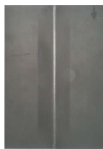
Electron Beam Welded AISI 4130 sample
