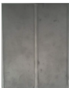
Electron Beam Welded AISI 1008 sample
