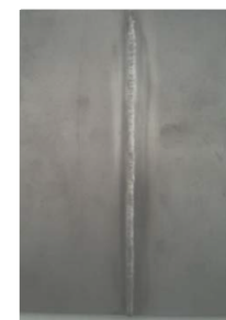
Tungsten Inert Gas Welded AISI 4130 sample
